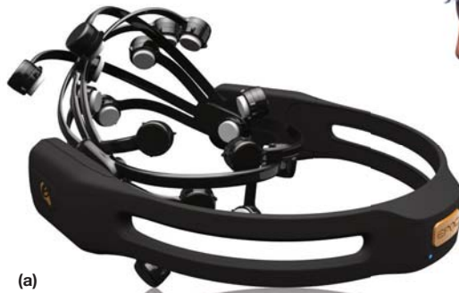
Figure 3 The Emotiv headset alone (a) and on a user (b) simplifies the acquisition of EEG signals by standardizing the placement of electrodes and by including proprietary algorithms that allow for differences in brain waves due to folds in the brain.
